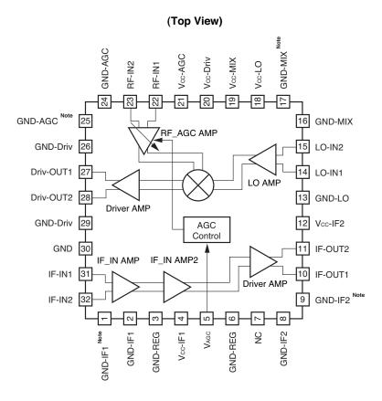
Note 1, 9, 17, 25-pin: Connected to the lead frame.
