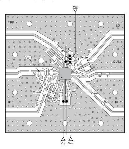
Note Balun Transformer : TOKO 617DB-1674 B4F (Double balanced type)
