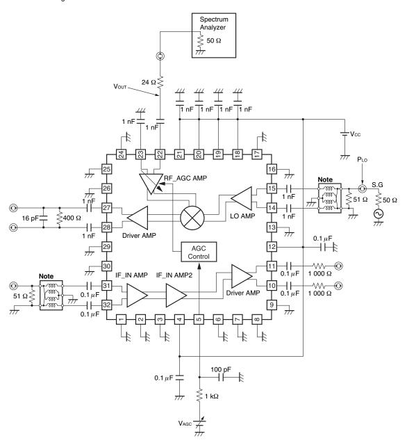
(frf = 70 to 130 MHz (frf = 49.1 MHz  $\pm$  0.6 MHz), fLO = 119 to 179 MHz, PLO = -10 dBm, Vout = 0.7 Vp-p (Single Ended))
